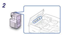
Clean the rollers (a total of three places) inside the feeder cover with a water-moistened cloth. Then, wipe the area with a soft, dry cloth.
